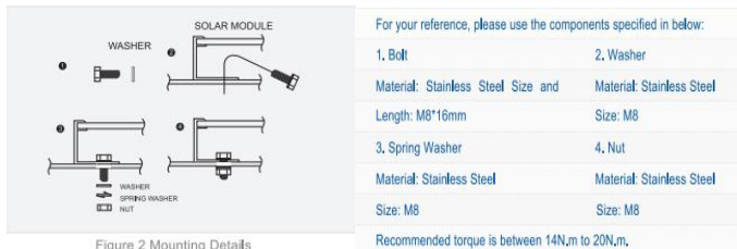
Figure 2 Mounting Details
